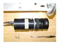
CCD camera – high field beam profile imaging
