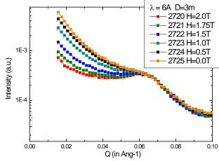
SANS scattering form the carpet (2D and after circular integration). Evolution of the signal as a function of the applied field. Task 4 (CEA, JCNS, TUD)
