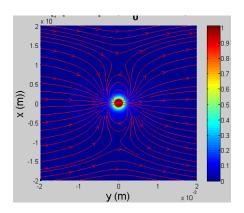
Magnetic induction field maps can be generated which include both the internal magnetization, the stray fields generated outside the magnetic object and the applied magnetic field
