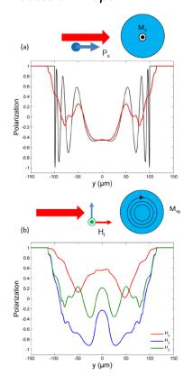
It is possible to plot the precession scan maps for various magnetic configurations and applied magnetic field.
