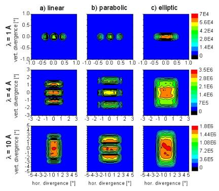
Fig. 7: Vertical and horizontal intensity distribution versus the divergence for wavelengths  $\lambda = 1 \text{ Å}, 4 \text{ Å}, 10 \text{ Å}$  of a) ballistic guide with linearly tapered divergent and convergent sections, b) ballistic guide with parabolic divergent and convergent sections, c) elliptic guide.
