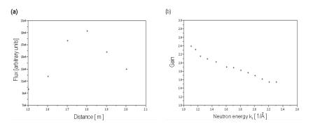
Fig. 5: (a) neutron intensity behind guide exit – focal point at 1.8 m after monochromator; (b) gain with focusing guide over a setup without trumpet for different neutron energies
