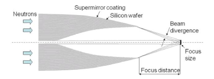
Such focusing lenses can be used for imaging purposes where i) cone beam geometry is used or ii) high-flux density in the focal point is used for high-spatial resolution experiments. •Test of solid state lenses was performed at the neutron imaging instrument CONRAD at HZB. The figure shows the neutron intensity behind the end of the lens, with the focus at 36mm.
