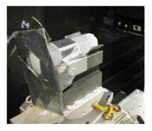
A focusing device based on Kumakhov-type lenses was used which focuses a cross-section of 2 cm into a diameter of less than 1mm provided a flux gain of 20x which was essential for the application of a high resolution detector with a pixel size of 2 µm. In this way realistic exposure times of several minutes were achieved.
