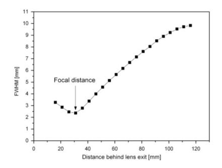
FWHM of the neutron intensity perpendicular to the beam direction in dependence of the distance from the end of the lens.
