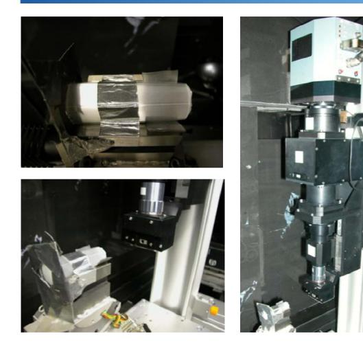
**High-resolution** neutron imaging setup. A Kumakhov lens is used to focus the beam at the scintillator screen. High resolution detector based on light microscope magnifies the image from the scintillator on the CCD chip providing effective pixel size of 2 µm. The setup was equipped with a GGG scintillator screen.
