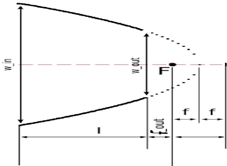
$f_{out}$  = distance from the exit of guide to second focal point
