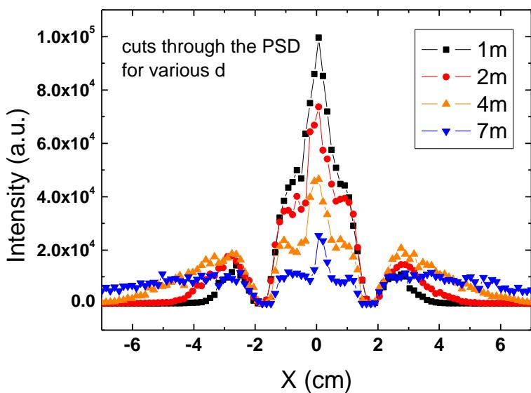
Intensity increases with increasing m value of the coating due to reflection of neutrons with higher angle of incidence
