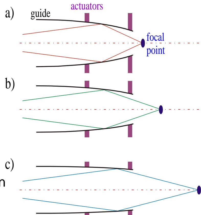
Adjust curvature of tapered guide by means of actuators
