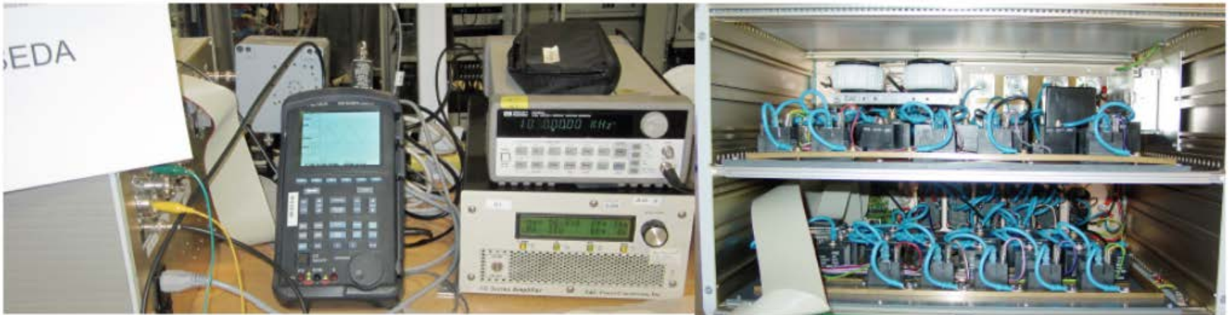
Fig. 1. The radio frequency generator, amplifier (left) and capacitors (right) used.
